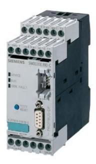
BASIC UNIT 1 SIMOCODE PRO C; PROFIBUS DP-INTERFACE 12 MBIT/S, RS485; 41/30 FREELY PARAMETERIZABLE; US: DC 24V; THERMISTOR MOTOR PROTECTION; OUTPUTS MONOSTABLE
