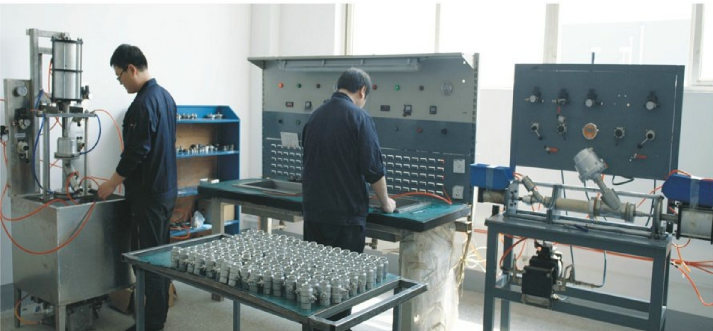
■ 阀门密封&性能检测 Valve Sealing & Functional Test
