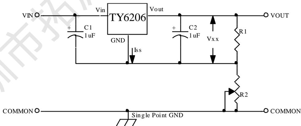
$$V_{out} = V_{xx}(1 + R_2/R_1) + I_{ss}R_2$$
