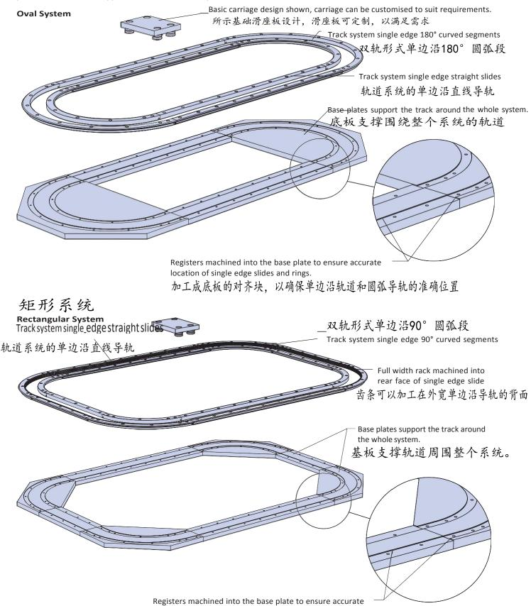
location of single edge slides and rings. 加工成底板的对齐块,以确保单边沿轨道和圆弧导轨的准确位置
